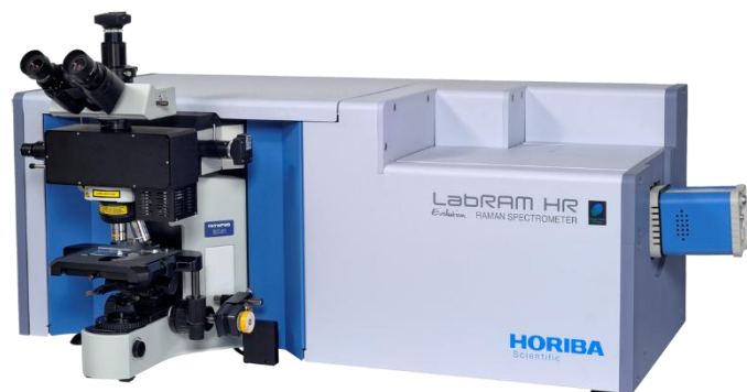
Figure 5. HORIBA LabRAM HR Evolution Confocal Raman Microscope.
