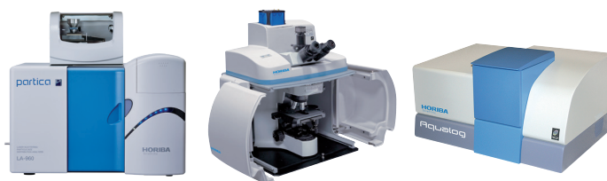
Figure 1. Experimental systems used for these experiments. Left: LA-960 Particle Size Analyzer. Middle: XploRA™Plus Raman micro-spectrometer. Right: Aqualog spectrofluorometer.
