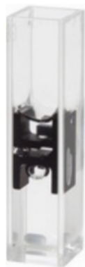
Figure 1. ViewSizer 3000 cuvette includes a black insert that houses a magnetic stir bar to keep larger particles suspended and mix the particles between videos.
