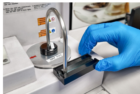
Figure 2. The sniffer tray sliding under the vacuum nozzle attached to the PowderJet.
