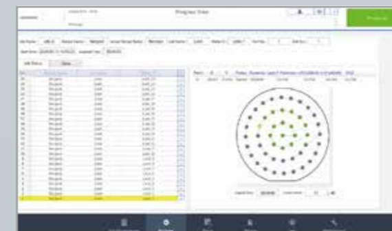
Measurement in progress: The progress of the measurement is indicated in yellow during measurement, green after measurement, and gray before measurement.
