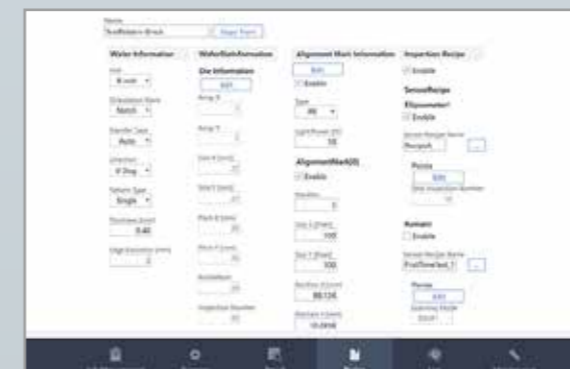
Recipe setting screen: Different sensors (spectroscopic ellipsometry, Raman spectroscopy, PL) can be operated from the same software platform
